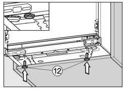
■ Screw in adjustable feet ② completely.
